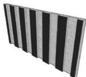
The parts of the wood wool board that are installed in direct contact with the base are fitted with vapor barriers.
